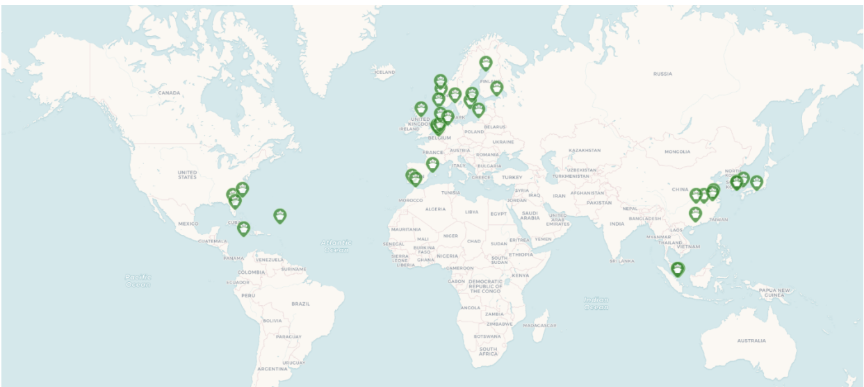
Figure 4-9 Current LNG bunkering infrastructure (from DNV AFI platform). Only bunkering vessels are shown.
