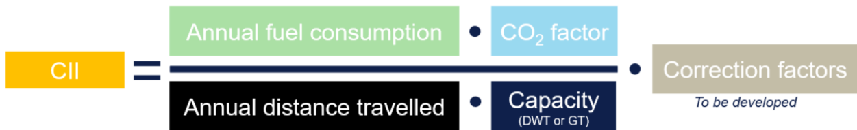
Figure 3-7 Calculation of CII. Correction factors and voyage exclusions to be developed in 2022.
